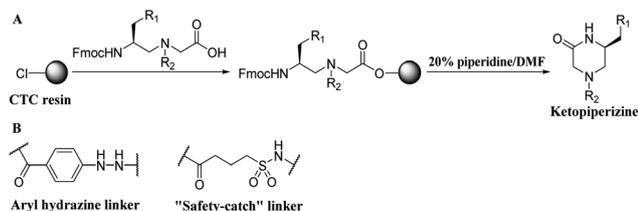
**Fig. 2** (A) Ketopiperazine formation, which prevents the sequence elongation. (B) Aryl hydrazine linker and 4-sulfamylbutyryl "safety-catch" linker used to eliminate ketopiperazine formation.
