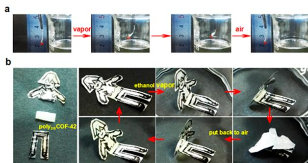
**Figure 7.** (a) Optical images of the  $\text{poly}_{2/6}\text{COF-42}$  membrane used as an artificial arm with a hanging red object. (b) Demonstration that the doll made from the  $\text{poly}_{2/6}\text{COF-42}$  membrane can perform a series of complicated movements (e.g., sit-ups) upon exposure to ethanol vapor or air.
